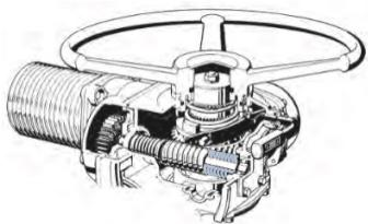
**Fail-safe spring actuators:** During powered operation the springs travel with the actuator. The actuator opens and closes the valve, and provides braking. Under loss of power, the spring is released and drives the actuator to the pre-designated fail-safe position.
