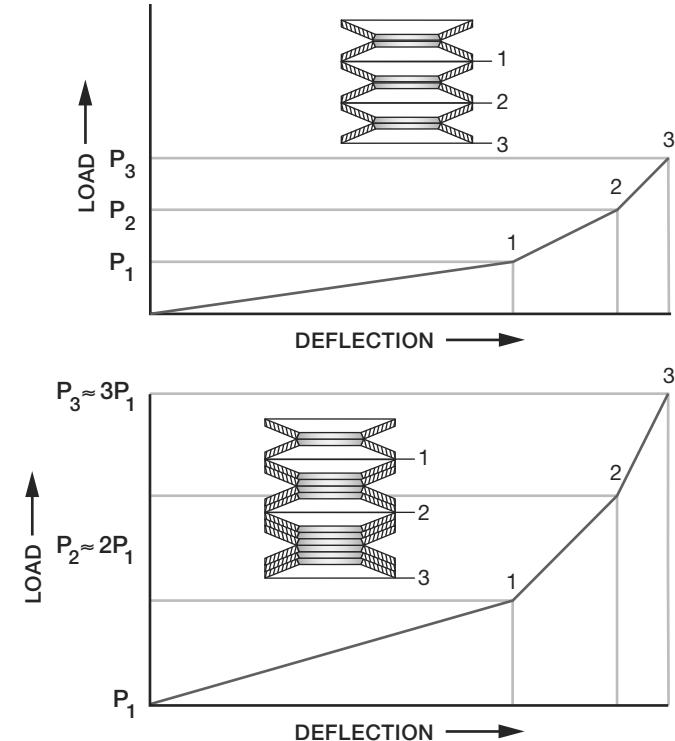
Disc springs of differing thickness can be stacked in series to obtain a progressively rising load. This effect is also obtained using same thickness springs, but incrementally increasing the units in the stack. Care must be taken not to over-stress the spring in the stack.
