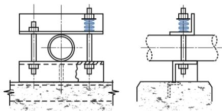
Long pipe runs require structural support, but are also subject to movement due to temperature changes. A structural support that includes disc springs can both support and control the pipe, by allowing some movement when required.
