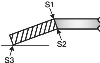
For evaluation of compressive stress, use formula S1. It computes the compressive stress at the upper inner diameter. This compressive stress may be as high as 400,000 psi for certain bolted applications.
