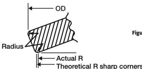
Typically, the overall height of the disc spring is specified because it is easy to measure and control. The cone height ( $h$ ), on the other hand, is difficult to measure (see Figure 4).
